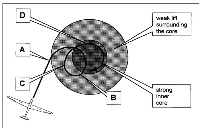
Figure 2 Thermal centering by varying angle of bank
