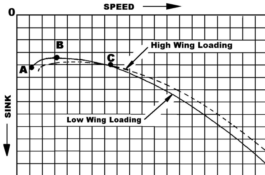
Figure 7 The polar curve (Speed polar)
