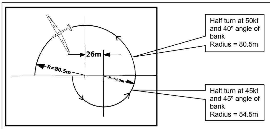
Figure 8 Re-positioning of a glider as a result of inaccurate flying
