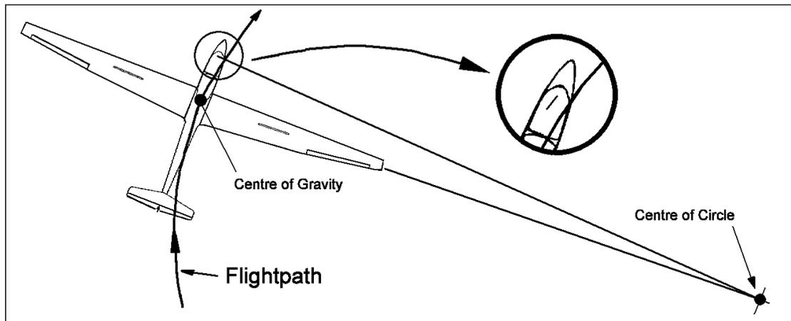
Figure 9 Use of "top rudder" for optimum thermalling performance
