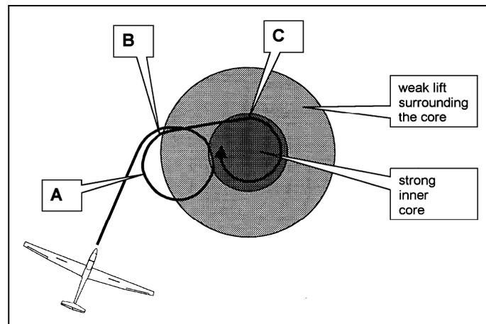
**Figure 3 Worst heading thermal centering method**
