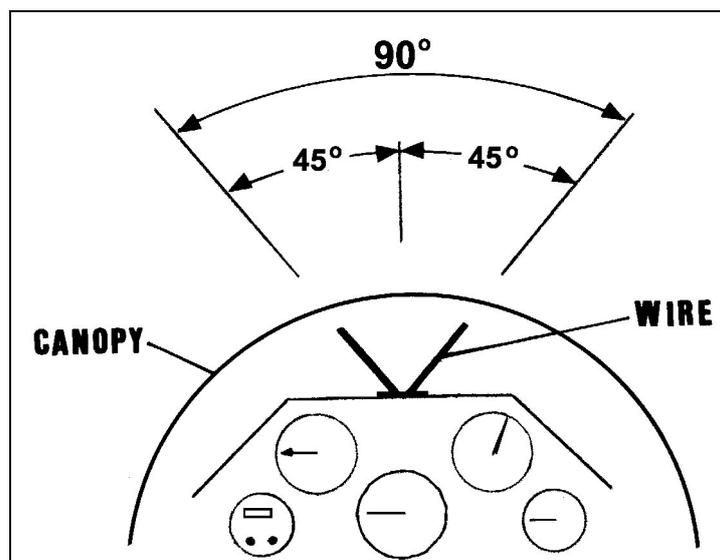
Figure 10 Angle of bank indicator
