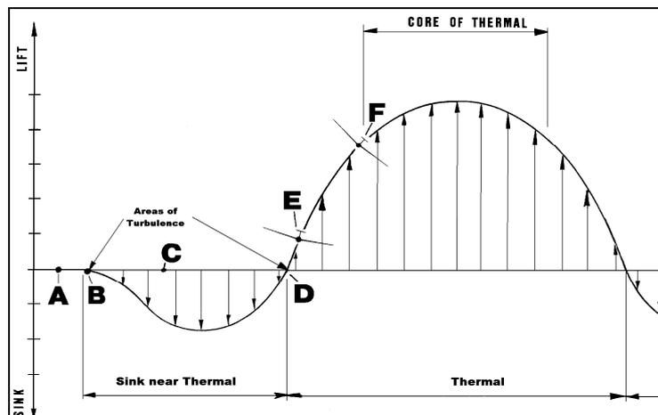
Figure 4 Vertical air movements (simplified)
