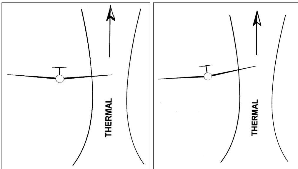
Figure 1 Lifting of wing by thermal (not to scale)
