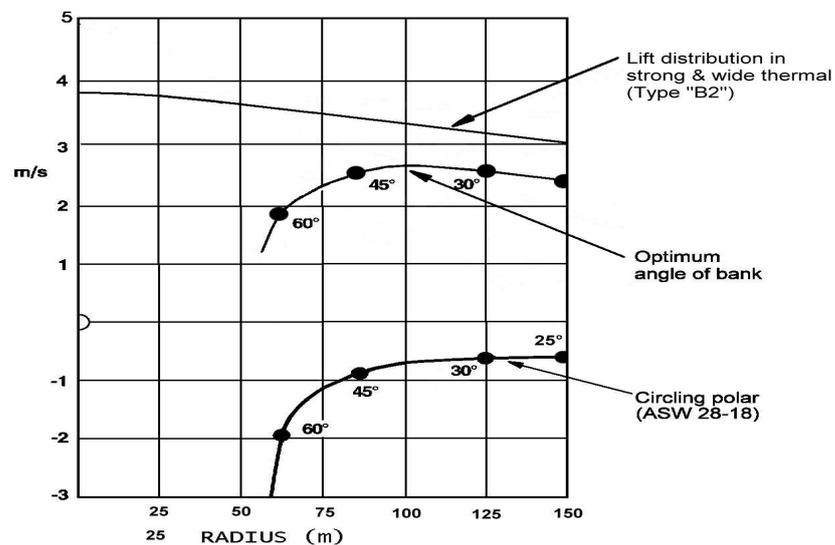
Figure 6 Optimum angle of bank for strong and wide thermal
